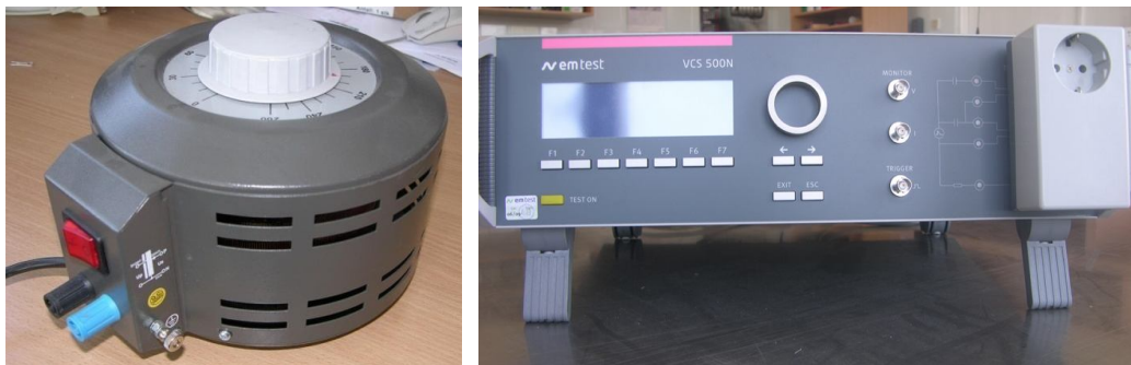
Fig. 10. Testing arrangement for supply voltage variation
