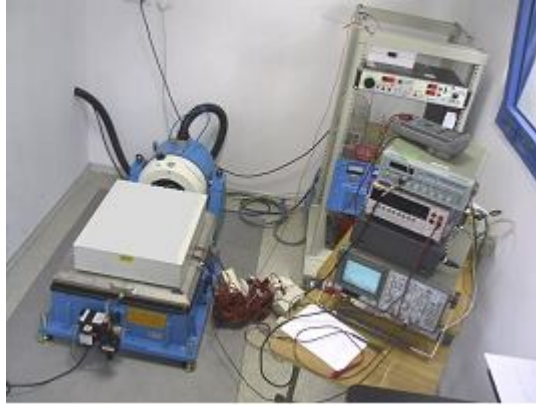
Fig. 9. The view of the shaker
