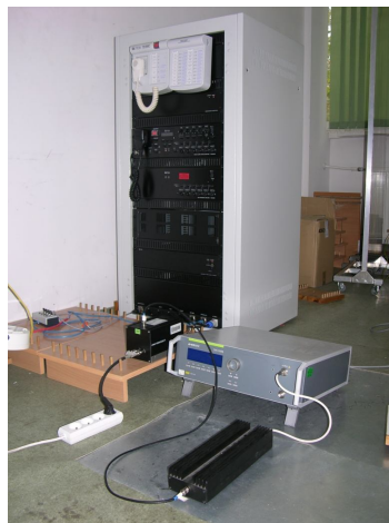
Fig. 13. Testing arrangement for the conducted disturbance induced by magnetic fields
