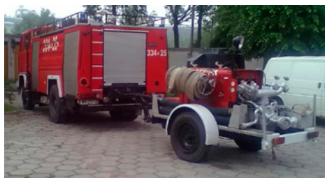
Rysunek 3. Samochód GCBA 5/32 wraz z motopompą M48/8 Figure 3. Heavy firefighting vehicle GCBA 5/32 with motor pump M48/8
