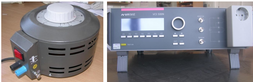
Fig. 10. Testing arrangement for supply voltage variation
