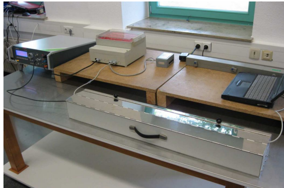
Fig. 14. Testing arrangement for fast transient burst
